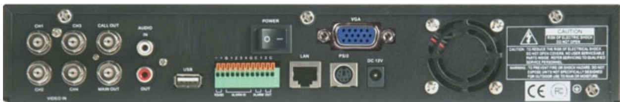
4CH-IN TV Audio USB ALARM LAN Mouse 12Vdc
