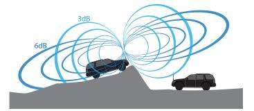
When operating between mountainous and open terrain, think about choosing an antenna with interchangeable high gain and low gain whip tops, or use two antennas with an RF switch.
