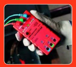
EPM3 Safe and simple go-no-go testing for phase sequence and motor rotation, see page 16
